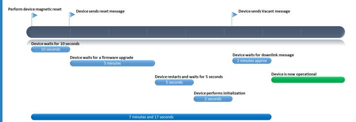
5. Once the device is done initialization, it will send a message frame denoting vacant status of the parking slot to the cloud, an example is shown below. The device will wait for downlink configuration, if any, and then start normal operation.
